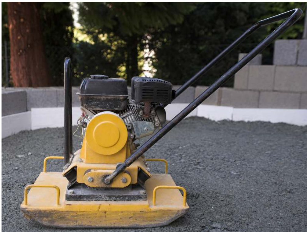
Motorn driver den tunga bottenplattan, vars vibrationer packar stenmaterialet. [73]
