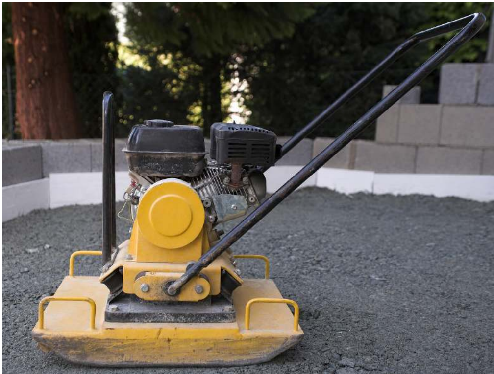
Figure 25. A vibrating plate compactor, often nicknamed a “frog” on site
